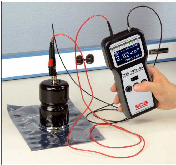
Figure 2. Using the Concentric Ring Probe with the SCS 770760 Resistance Pro Meter
