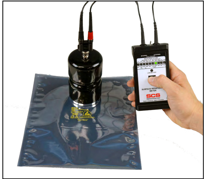
Figure 4. Using the Concentric Ring Probe with the SCS SRMETER2 Surface Resistance Meter
