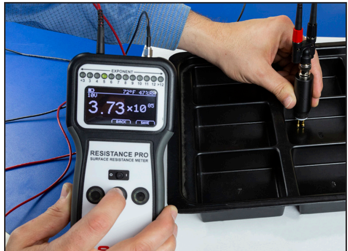
Figure 2. Using the Two-Point Resistance Probe with the SCS 770760 Resistance Pro Meter Kit
