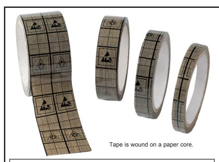
ANSI/ESD S20.20 requires that all nonessential insulators, such as those made of plastics and paper, must be removed from the workstation. Substituting ESD tape for regular tape (a very high tribocharging insulator) protects your ESD susceptible products.
