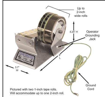
\*Best practice is grounding via supplied ground cord. Attach cord to snap on chassis and to common point ground. If grounded via placing on a grounded ESD worksurface, resistance to ground (RTG) should be periodically tested <1 x 10E9 ohms.
