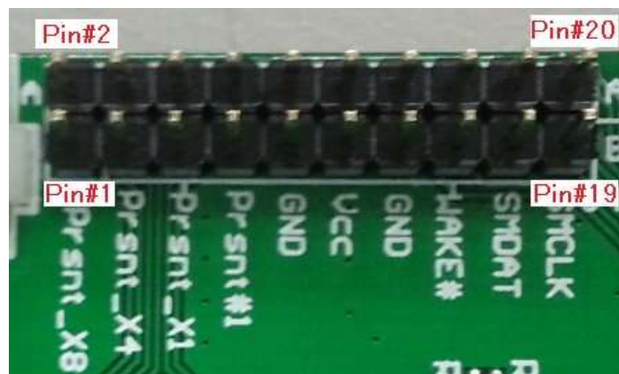
Figure-3: J4 pin header for PCIe side-band signal
