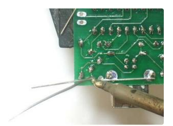
Solder and clip the two LEDs.
