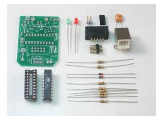
Check the kit to verify you have all the parts necessary (the 0.1uF capacitor is missing, oops!).
