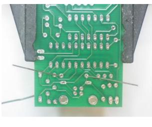
Bend the wire legs so that when the board is flipped over, it won't fall out.
