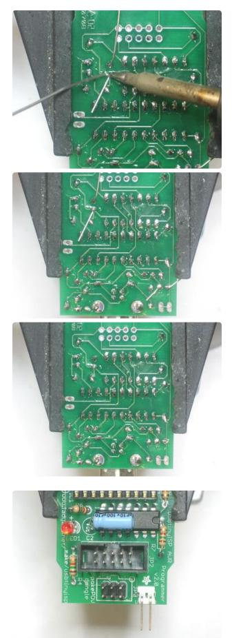
Solder and clip both capacitor's leads.
