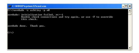
You should get that response, which means that it communicated with the programmer but failed to find a connected chip.
