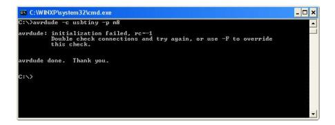
This response from avrdude means that it can talk to the programmer but the programmer can't talk to the chip.
