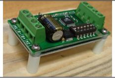
Figure 2.3: Mounted to a wood frame using standoffs
