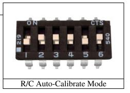
the minimum and maximum control inputs, and use those to set the control range. If the driver is initialized with the control stick at either extreme, the driver will operate in single-direction mode.
