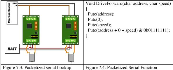
Example: So in this function, if address is 130, command is 0 (for driving forward), speed is 64, the checksum should calculate as follows:
