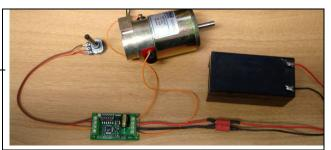
The 5V terminal can be used to power small loads, like a potentiometer or a radio receiver. The 0V signal must be connected to the ground of the device generating the input signal.
