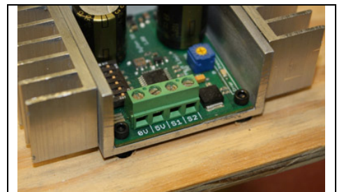
Figure 2.3: Mounted to a wood frame using standoffs
