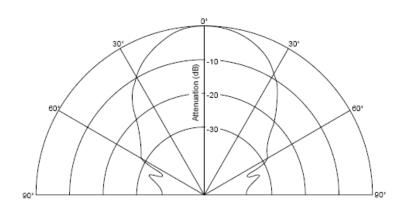
Figure 1: URM04 Beam Width 60 degree
