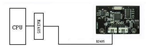
Figure 4 Connect Sensor to MCU via MAX485
