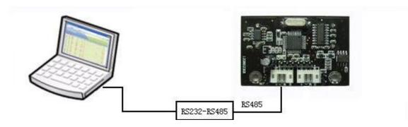
Figure 6 Connect Sensor to PC via RS232-RS485 Converter
