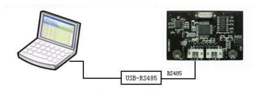
Figure 5 Connect Sensor to PC via USB-RS485 converter
