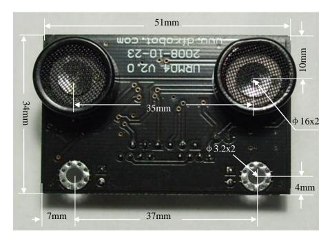
Figure 2: URM4 V2 front view and dimension
