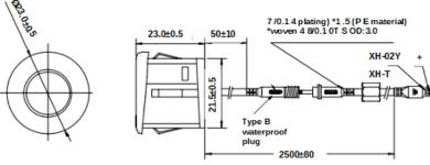
**Note:** Dimension for "K" and "W" are not applicable on MB8460/MB8480 CarSonar-WR sensors. The recommended operating and storage temperature of the CarSonar-WR is –40C to +75C.
