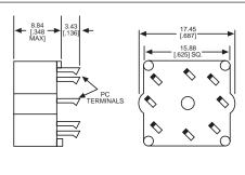
Material: All plastic switch components made from 94V-0 plastic
