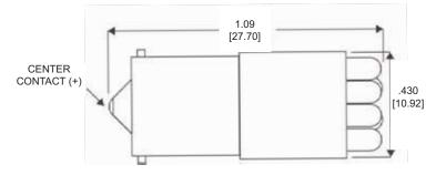
Measurements are typical Dimensions are inches [mm]
