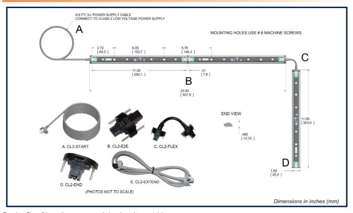
Requires Class 2 low voltage power supply (purchased separately) Total power consumption of modules should not exceed rating of power supply Observe minimum rating of power supply used
