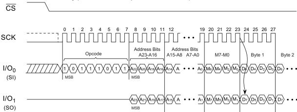
Figure 7-4. Dual-I/O Fast Read Array (Initial command or previous M5, M4  $\neq$  1,0)
