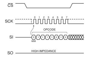
Figure 8-7. Erase/Program Resume Command Timing
