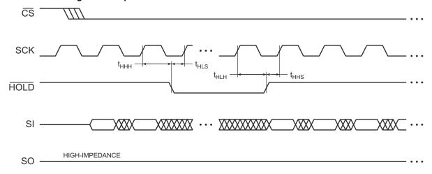
Figure 14-5. HOLD Timing – Serial Output
