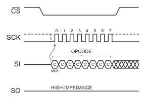
Figure 8-5. Chip Erase Timing
