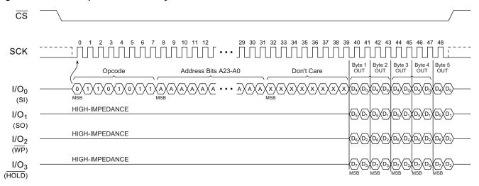
Figure 7-6. Quad-Output Fast Read Array
