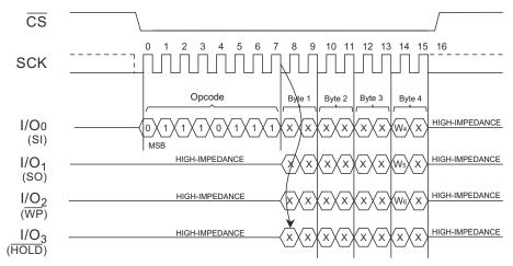
The Set Burst with Wrap instruction sequence is:  $\overline{CS}$  goes low  $\to$  Send Set Burst with Wrap instruction  $\to$  Send 24 Dummy bits  $\to$  Send 8 "Wrap bits"  $\to$   $\overline{CS}$  goes high.
