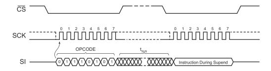
Figure 8-6. Erase/Program Suspend Timing
