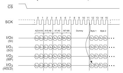
Figure 7-8. Quad I/O Read Array with Continuous Read Mode (Previous Command Set M5, M4 = 1,0)
