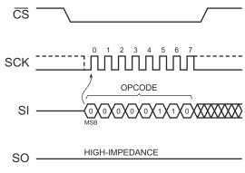
Figure 9-1. Write Enable Timing
