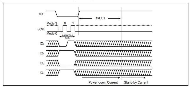
Figure 7-41. Release Power Down / Device ID Instruction (SPI Mode)
