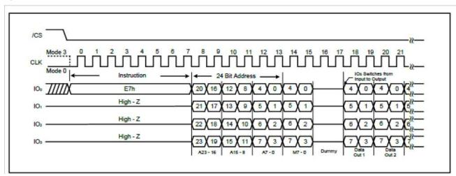
Figure 7-50. Word Read Quad I/O instruction (Initial instruction or previous set M7-0 ≠ Axh, SPI Mode)
