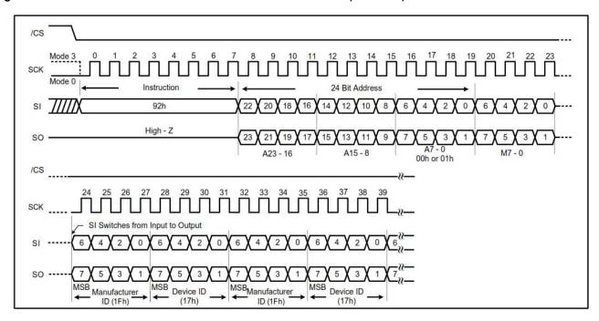
Figure 7-44. Read Dual Manufacturer/ Device ID Dual I/O instruction (SPI Mode)
