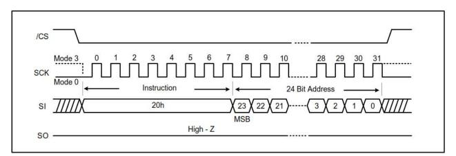
Figure 7-26. Block Erase Instruction (SPI Mode)
