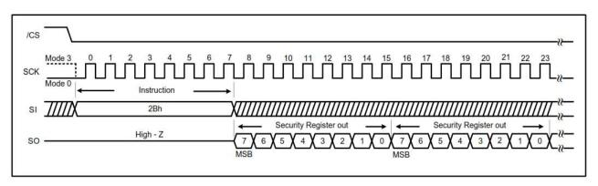
Figure 7-62. Read Security Register instruction (QPI Mode)
