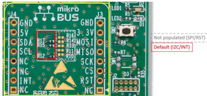
Figure 16: Default programming interface of MikroBUS™ module on DA14531 SMARTBOND TINY™ MODULE DB
