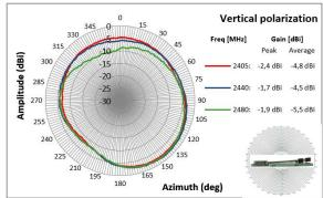
Figure 16: Radiation Pattern for XY-Plane, Vertical Polarization
