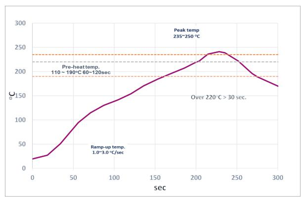
Figure 21: Recommended Reflow Profile for Lead Free Solder
