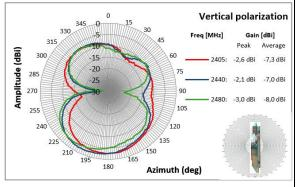
Figure 18: Radiation Pattern for XZ-Plane, Vertical Polarization
