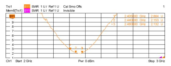
Figure 13: VSWR with Module Installed in the Upper Right Corner (Position #3) of the Evaluation Board
