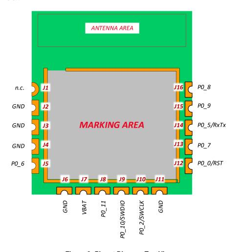
Figure 2: Pinout Diagram Top View
