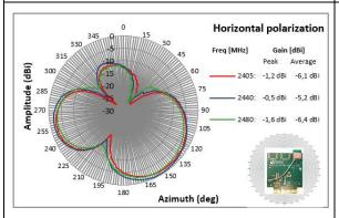
Figure 19: Radiation Pattern for YZ-Plane, Horizontal Polarization
