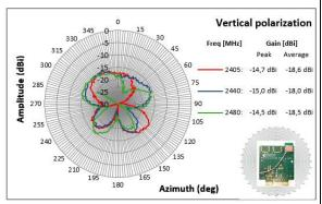
Figure 20: Radiation Pattern for YZ-Plane, Vertical Polarization
