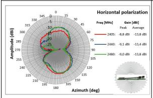
Figure 15: Radiation Pattern for XY-Plane, Horizontal Polarization
