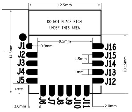
**Figure 4: Module Footprint Top View**
