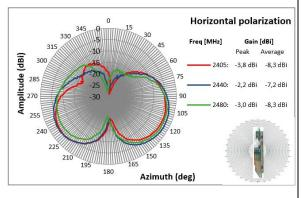
Figure 17: Radiation Pattern for XZ-Plane, Horizontal Polarization
