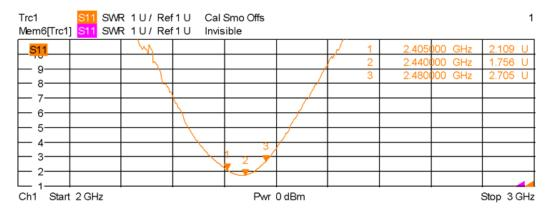
Figure 12: VSWR with Module Installed in Center (Position #2) of the Evaluation Board
