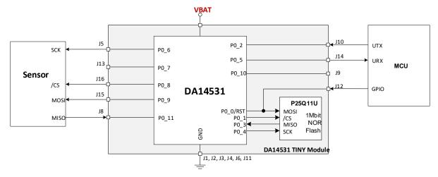
Figure 11: Example of Connecting a Sensor to the SPI Bus and an MCU to RST and UART
