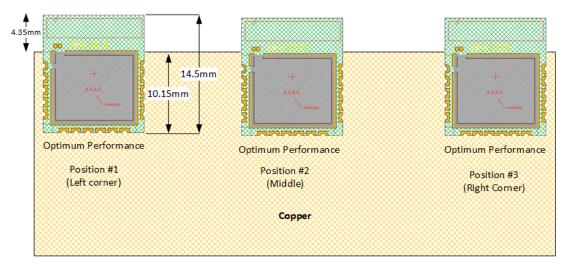
Figure 8: Installation Locations for Optimum Antenna Performance
