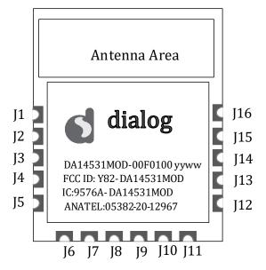
Figure 5: Module Shield Marking
