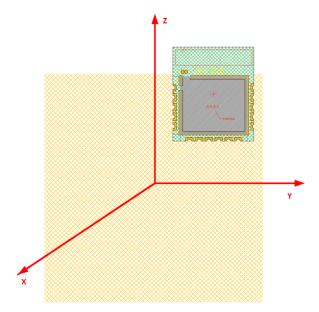
**Figure 14: Measurement Plane Definition**
