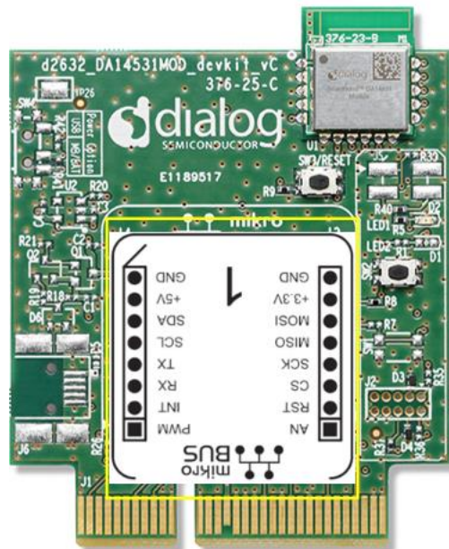
Figure 18: Example of mounting MikroBUS™ module
