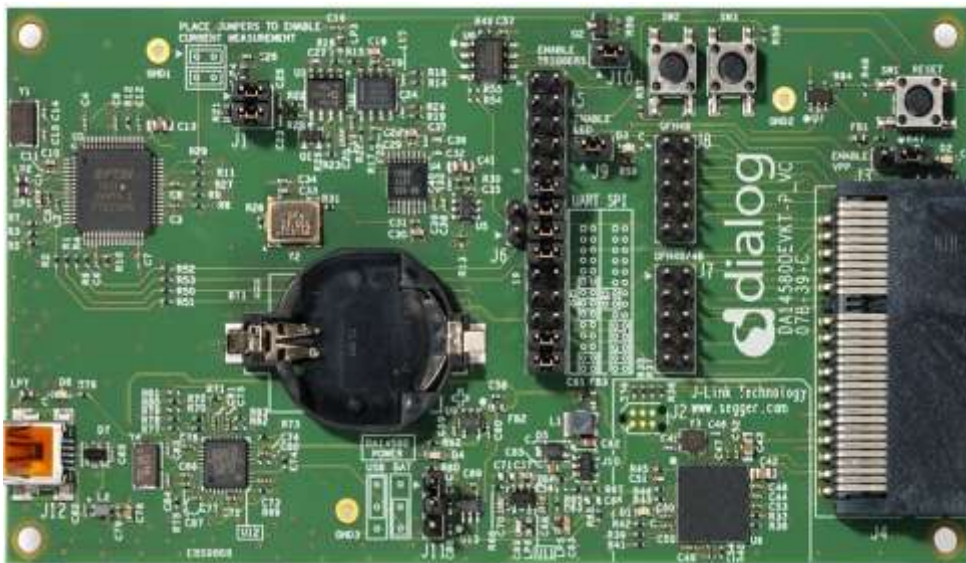
Figure 1: The DA14585/586 ProDev Kit Motherboard
