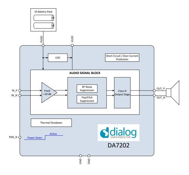
Figure 1: DA7202 block diagram
