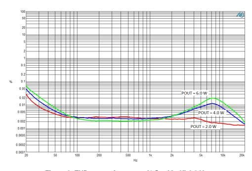
Figure 8: THD versus frequency (4  $\Omega$  + 33  $\mu$ H) 8.2 V
