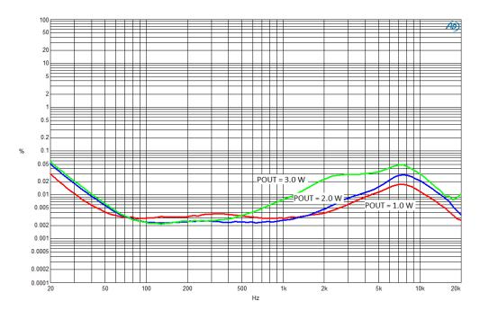
Figure 6: THD versus frequency (4  $\Omega$  + 33  $\mu$ H) 4.5 V
