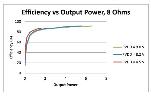
Figure 13: Efficiency versus output power (8  $\Omega$  + 33  $\mu$ H)
