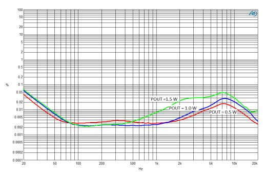
Figure 5: THD versus frequency (8  $\Omega$  + 33  $\mu$ H) 4.5 V
