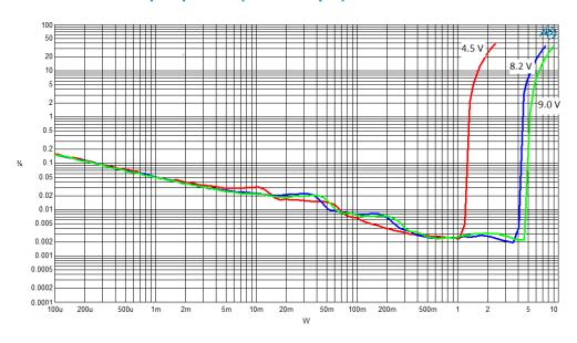
Figure 3: THD versus output power (8  $\Omega$  + 33  $\mu$ H)
