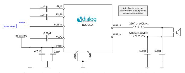
Figure 20: Layout of recommended external components and their values
