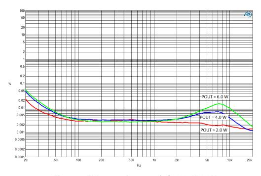
Figure 10: THD versus frequency (4  $\Omega$  + 33  $\mu$ H) 9.0 V
