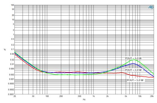
Figure 7: THD versus frequency (8  $\Omega$  + 33  $\mu$ H) 8.2 V
