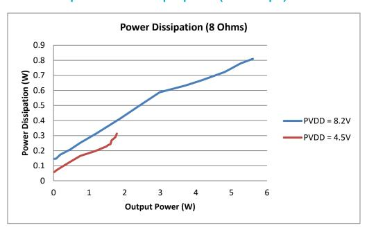
Figure 17: Power dissipation versus output power (8  $\Omega$  + 33  $\mu$ H)
