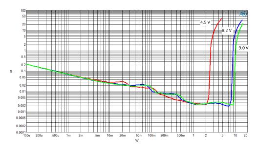
Figure 4: THD versus output power (4  $\Omega$  + 33  $\mu$ H)
