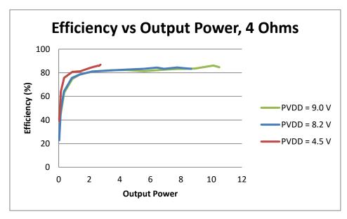
Figure 14: Efficiency versus output power (4  $\Omega$  + 33  $\mu$ H)
