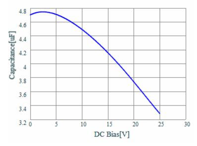
Figure 21: Performance plot of the sample capacitor used in the example (below)
