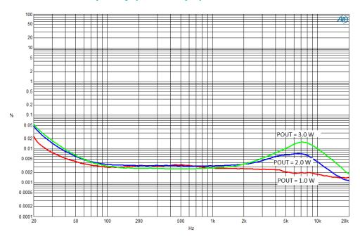
Figure 9: THD versus frequency (8  $\Omega$  + 33  $\mu$ H) 9.0 V
