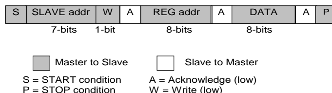
Figure 27: I 2 C Byte Write (SDA signal)
