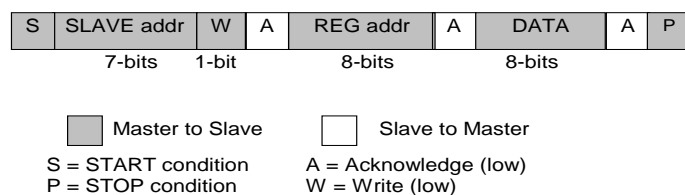
Figure 27: I 2 C Byte Write (SDA signal)
