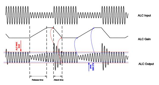
Figure 10: ALC Principle of Operation
