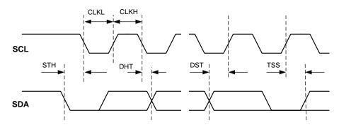
Figure 4: I<sup>2</sup>C Bus Timing
