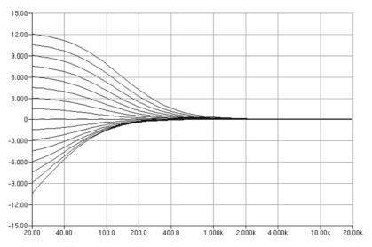
Figure 13: Equalizer Filter Band 1 Frequency Response at FS = 48 kHz
