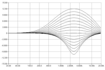
Figure 16: Equalizer Filter Band 4 Frequency Response at FS = 48 kHz
