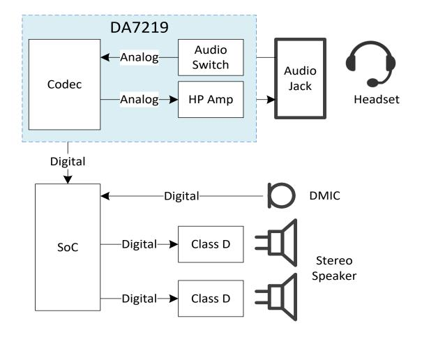
Figure 1: DA7219 in a Digital Distributed System
