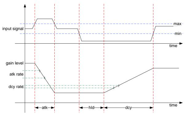
Figure 11: Attack, Delay and Hold Parameters
