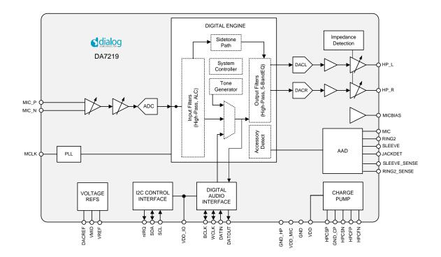
Figure 2: DA7219 Block Diagram
