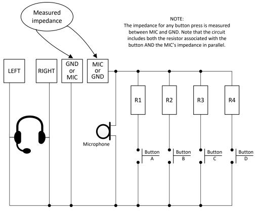
Figure 21: Measuring the Impedance of a Button Press
