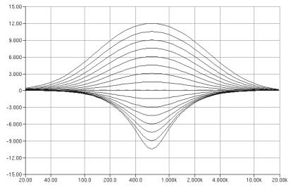
Figure 15: Equalizer Filter Band 3 Frequency Response at FS = 48 kHz
