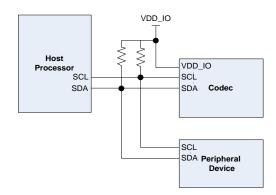
Figure 22: Schematic of the I<sup>2</sup>C Control Interface Bus
