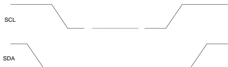
Figure 34: I 2 C START and STOP Conditions
