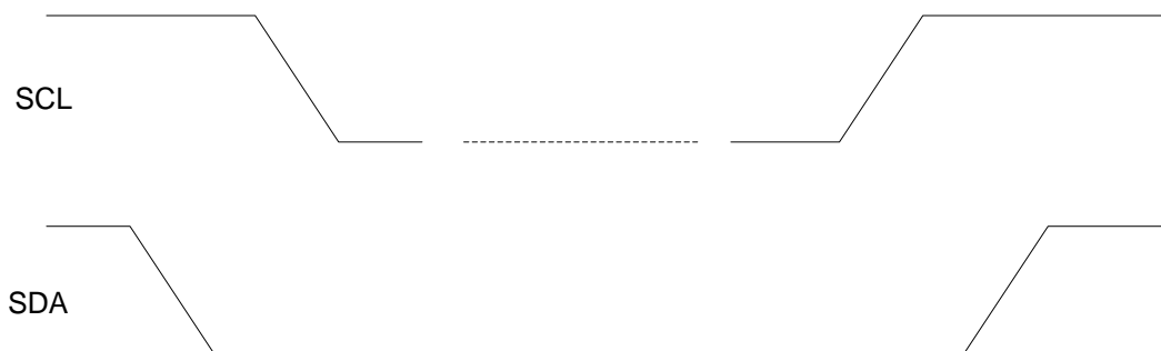
Figure 18: I 2 C START and STOP Condition Timing
