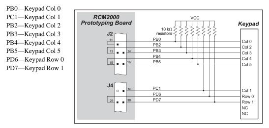
Connect the keypad to Parallel Ports B, C, and D.
