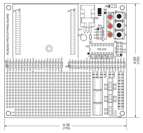
Figure B-2. RCM2000 Prototyping Board Dimensions
