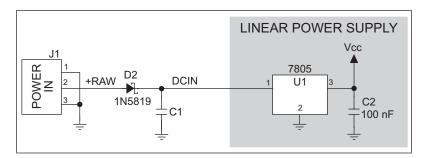
Figure B-3. Prototyping Board Power Supply
