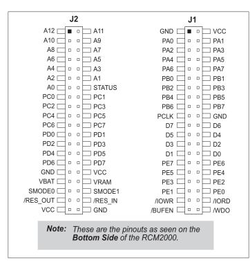
Figure 5. RCM2000 Pinout
