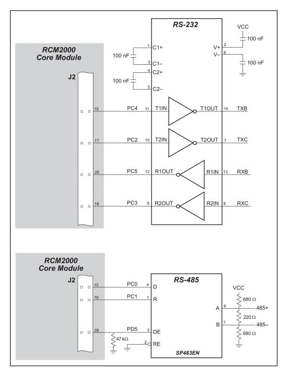
Figure D-1. Sample RS-232 and RS-485 Circuits
