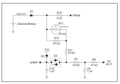
Figure C-2. RCM2000 Battery-Backup Circuit
