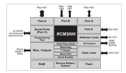
Figure 4 shows the subsystems designed into the RCM2000.
