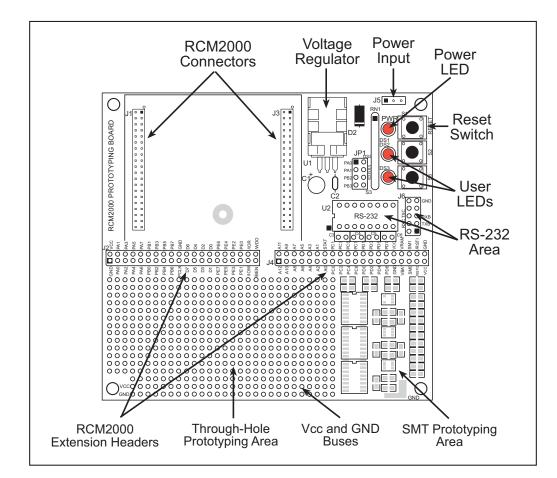
The Prototyping Board is shown in Figure B-1 below, with its main features identified.
