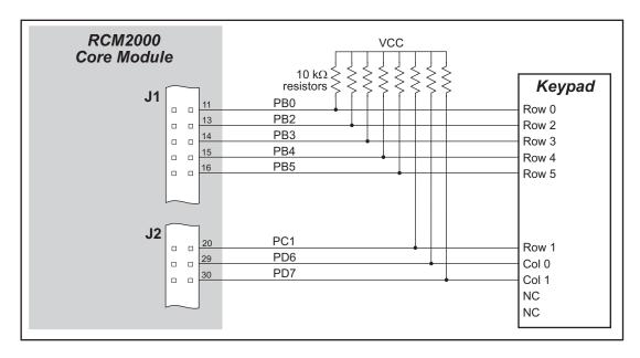
Figure D-2. Sample Keypad Connections
