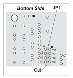
Figure B-4. Where to Cut Traces to Permanently Disable Demonstration Hardware on Prototyping Board
