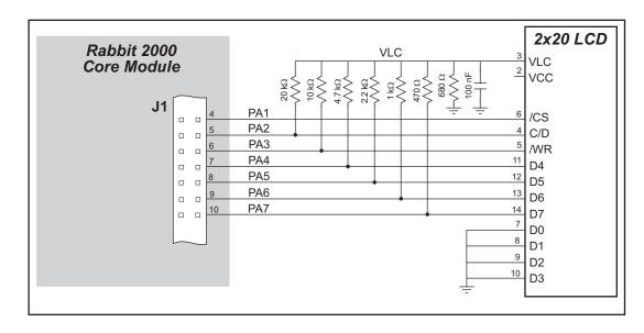
Figure D-3. Sample LCD Connections
