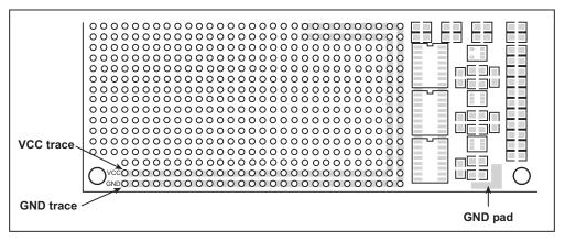
Figure B-6. VCC and GND Traces Along Edge of Prototyping Board
