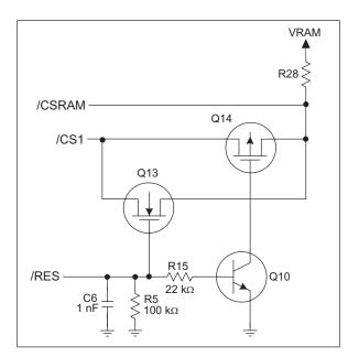
Figure C-4. Chip Select Circuit
