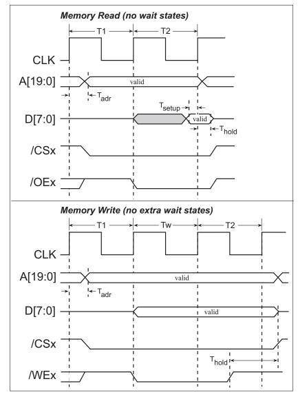
Figure A-4. Memory Read and Write Cycles
