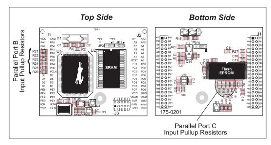
Figure 6. Locations of Digital Input Pullup Resistors
