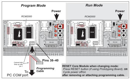
Figure 7. RCM2000 Program Mode and Run Mode Setup
