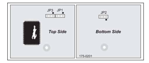
Figure A-6. Location of RCM2000 Configurable Positions
