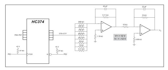
Figure D-6. Sample D/A Converter Connections
