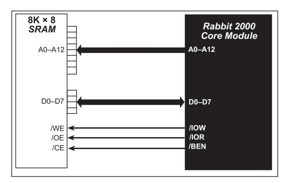
Figure D-5. Sample External Memory Connections
