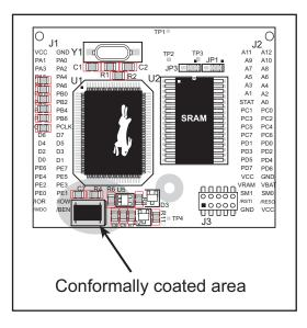
Figure A-5. RCM2000 Areas Receiving Conformal Coating
