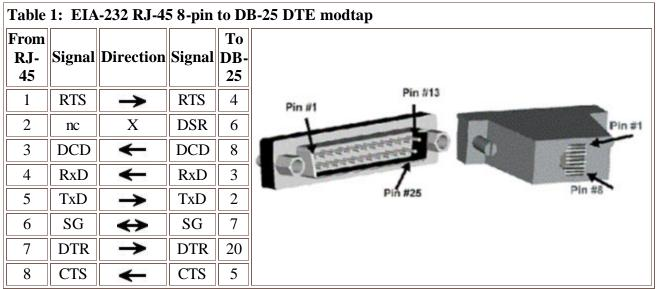
\* Arrows indicate which direction the signal is flowing
