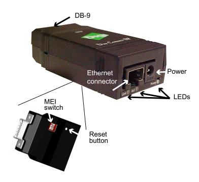
**Note:** MEI switches and the Reset button are in the same location for both the Digi Connect SP and Digi Connect Wi-SP.
