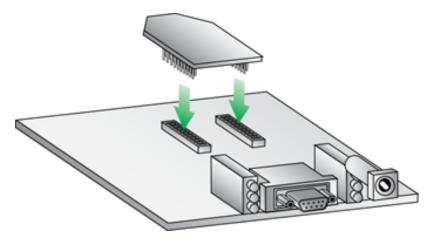
Century Interconnect and Samtec manufacture the  $2 \times 10$  pin 2 mm spacing receptacles on Digi development boards. Several other manufacturers provide comparable mounting solutions; we currently use the following receptacles:
