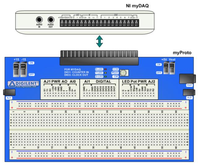
Figure 1. Connecting Digilent myProto to the NI myDAQ.
