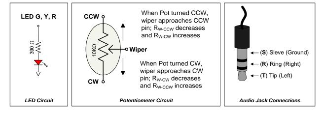
Figure 2. Digilent myProto circuits and breadboard device connections.
