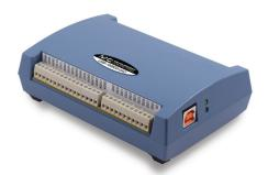
USB-1608G Series provides eight differential or 16 single-ended analog inputs, two analog outputs (USB-1608GX-2AO), 8 digital I/O, and one counter input.
