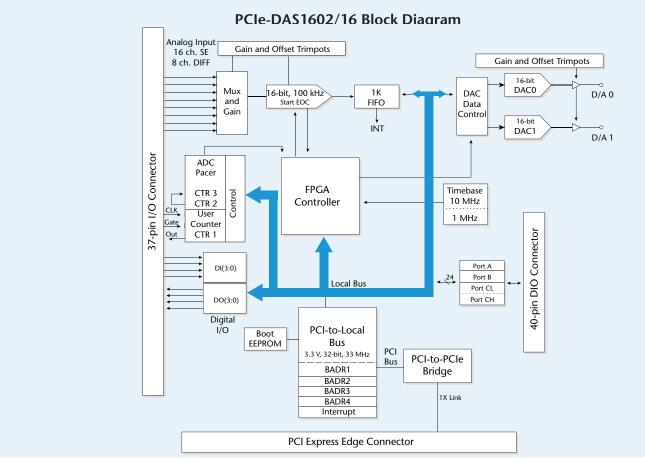
The eight digital I/O connections available on the main 37-pin connector consist of two 4-bit ports. One port is permanently configured as input, and the other port is permanently configured as output.
