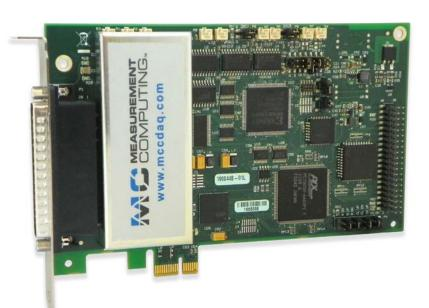
*The PCIe-DAS1602/16 provides 16 single-ended or eight differential analog inputs, sample rates up to 100 kS/s, two 12-bit analog outputs, 32 digital I/O, and three 16-bit counters*
