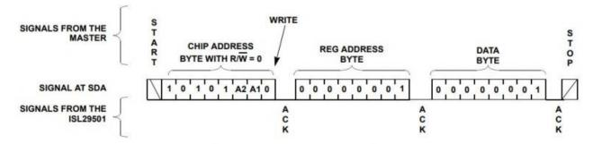
Example single-byte write sequence to the Pmod ToF
