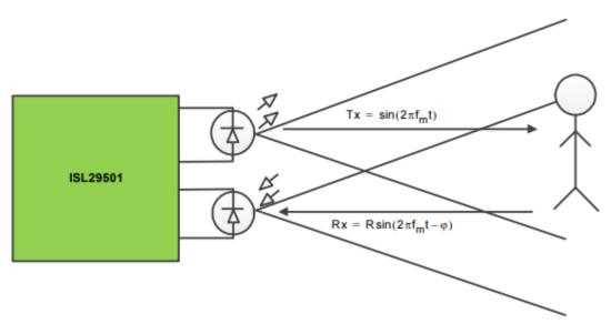
A measurement cycle of Pmod ToF is triggered by a falling edge on the sample start (SS) pin, or by the host board issuing a soft\_start to the ISL29501's command register via I2C. When performing a measurement, the chip emitter driver transmits a modulated square wave (Tx) at a given frequency optical signal (fmodfmod) through the emitter. The received optical signal (Rx) returns with a phase shift and attenuation depending on
