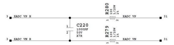
Figure 14 - Anti-Aliasing Filters for XADC Inputs
