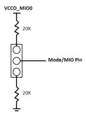
Figure 15 - Configuration Mode Jumpers
