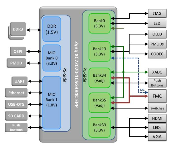
Figure 2 - Zyng Z7020 CSG484 Bank Assignments
