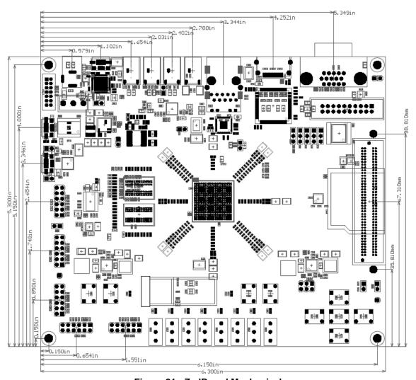
Figure 21 - ZedBoard Mechanical
