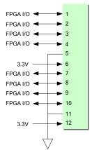
**Figure 12 - Pmod Connections**
