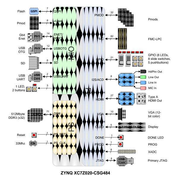
Figure 1 - ZedBoard Block Diagram
