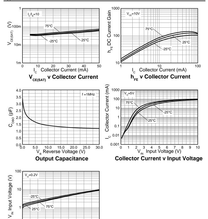
**Input Voltage v Collector Current**
