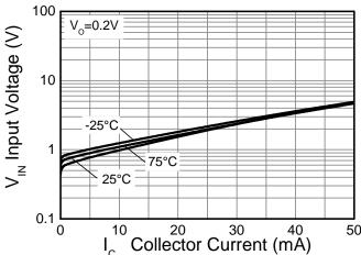
Input Voltage v Collector Current
