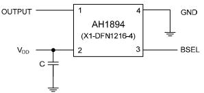
4. C<sub>IN</sub> is for power stabilization and to strengthen the noise immunity, the recommended capacitance is 100nF typical. Note:
