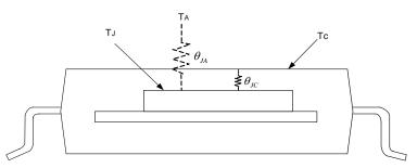
Notes: 5.  $\theta_{JA}$  should be confirmed with what heat sink thermal resistance. If no heat sink contacting,  $\theta_{JA}$  is almost the same as  $\theta_{JC}$ .
