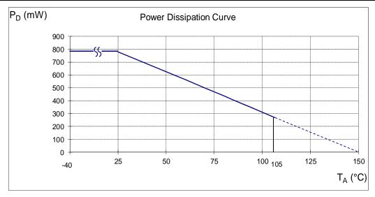
Notes: 11. DFN2020C-6 exposed pad soldered to minimum recommended landing pads (see Package Outline Dimension section) on a two-layer 2oz. copper FR4 PCB (1.6mm thickness) with no thermal vias in exposed PADs or any copper flood connecting to the landing pattern of the exposed pad.
