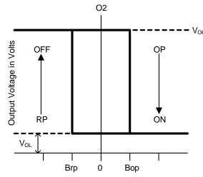
Magnetic Flux Density in Gauss
