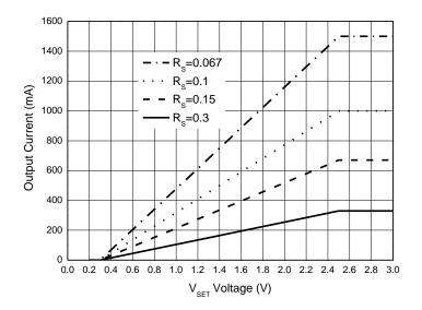
Figure 1. Analog Dimming Curve
