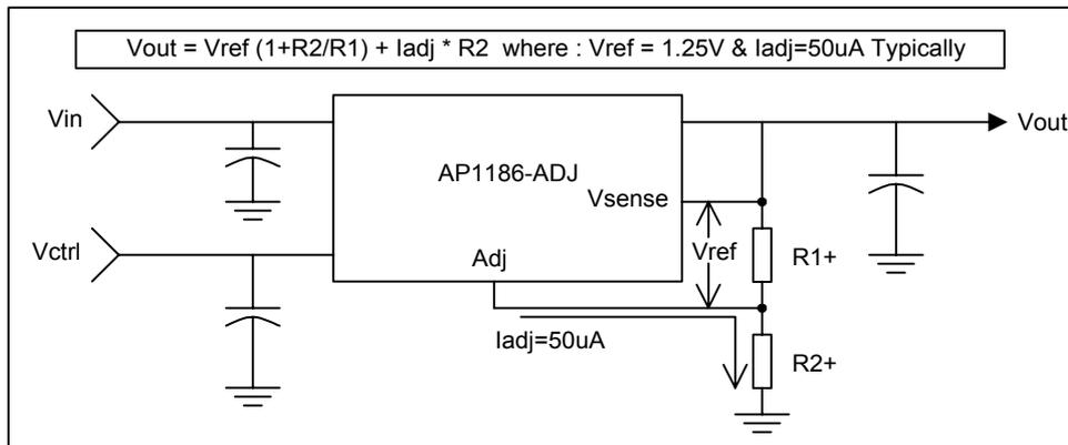
The AP1186-ADJ keeps a constant 1.25V between the Vsense pin and the Adj pin. By placing a resistor R1 across these two pins and connecting the Vsense and Vout pin together, a constant current flows through R1, adding to the Iadj current and into the R2 resistor producing a voltage equal to the  $(1.25/R1) * R2 + Iadj * R2$ . This voltage is then added to the 1.25V to set the output voltage. This is summarized in the above equation.
