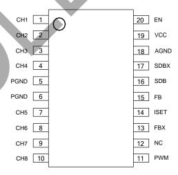
Note: AGND must be quiet and directly connected to total  $C_{\mbox{\scriptsize IN}}$
