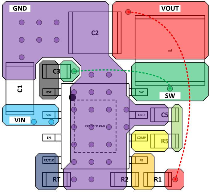
Figure 32. Recommended PCB Layout
