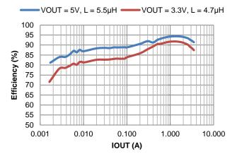
Figure 4. Efficiency vs. Output Current, VIN = 12V
