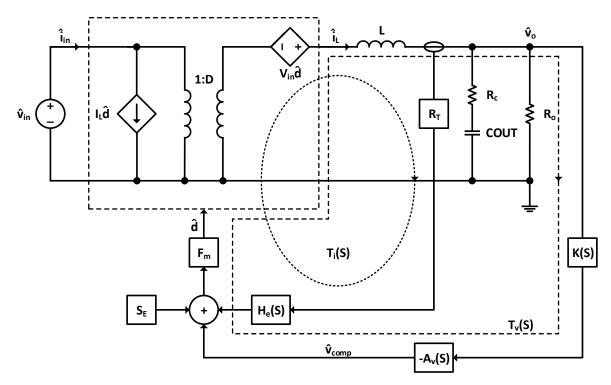
Figure 26. Small Signal Model of Buck Regulator
