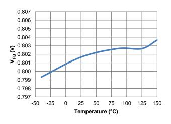
Figure 8. Feedback Voltage vs. Temperature
