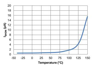
Figure 11. ISHDN vs. Temperature
