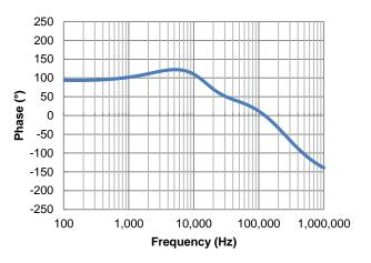
Figure 31. Closed-Loop Phase Margin
