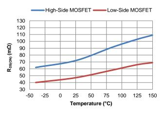
Figure 9. Power MOSFET RDS(ON) vs. Temperature
