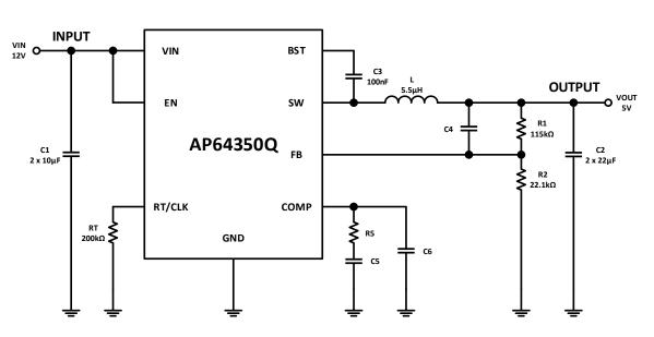
Figure 28. Example Circuit for Loop Compensation Calculations
