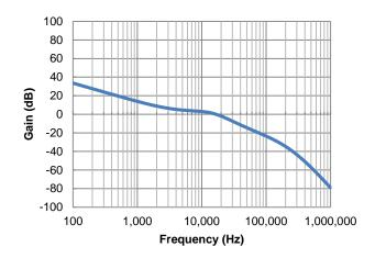
Figure 30. Closed-Loop Bandwidth
