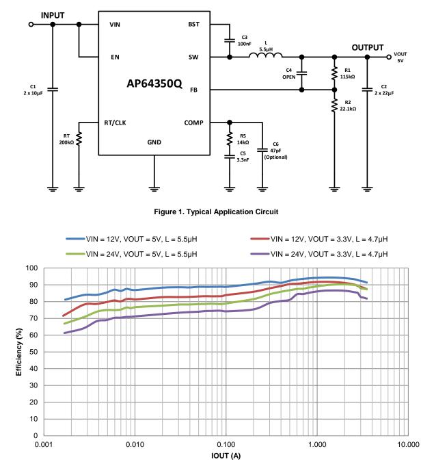
Figure 2. Efficiency vs. Output Current
