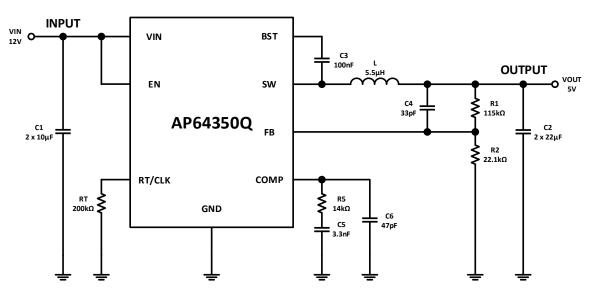
Figure 29. Example Circuit with Calculated Component Values for Loop Compensation
