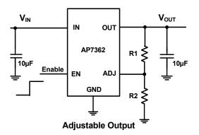
The output voltage is calculated by:
