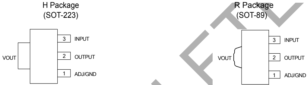
Figure 2. Pin Configuration of AZ1117B (Top View)
