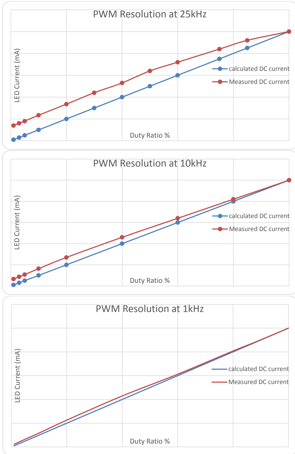
Figure 4. Typical LED Current Response vs. PWM Duty Cycle for 25kHz, 10kHz and 1kHz PWM Frequency (Refer to Circuit 3b)
