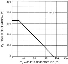
Figure 1 Power Derating Curve, Total Package
