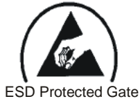
ESD Protected Gate
