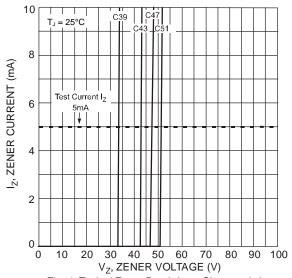
Fig. 4 Typical Zener Breakdown Characteristics
