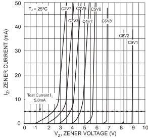
Fig. 2 Typical Zener Breakdown Characteristics
