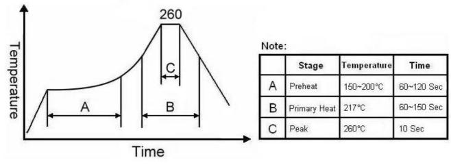
For soldering reflow profile and reliability test ratings go to: http://www.pericom.com/pdf/sre/reflow.pdf
